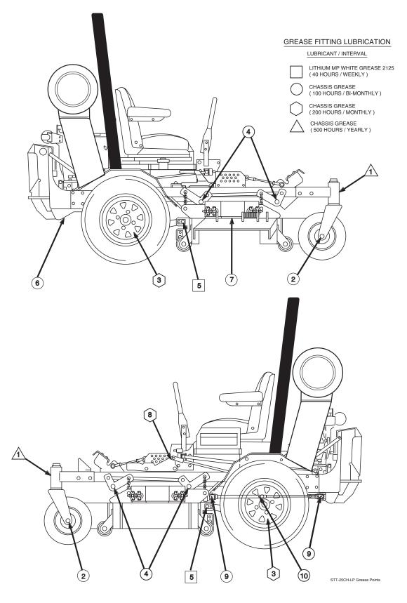
Figure 7-1. Lubrication Fitting Points
